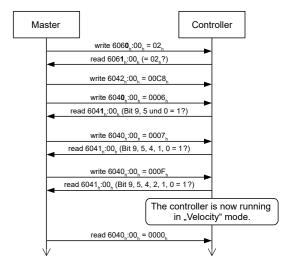
4. To stop the motor, set controlword (6040<sub>h</sub>) to "0".
