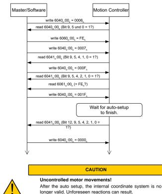
Restart the device after an auto setup. Homing alone does not suffice.
